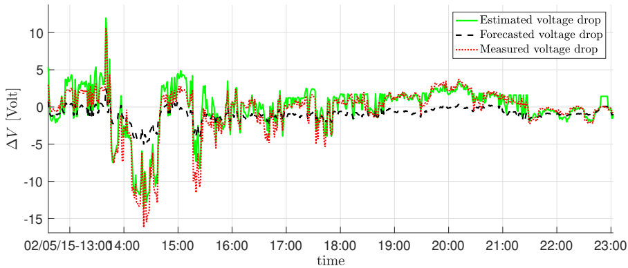
Figure 4.8: Comparison of forecasted and estimated voltage with real voltage measurement at the Neighborhood Battery bus.
